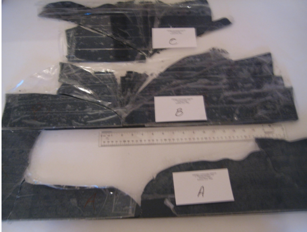
Break patterns of three samples of spandrel glass fracture
