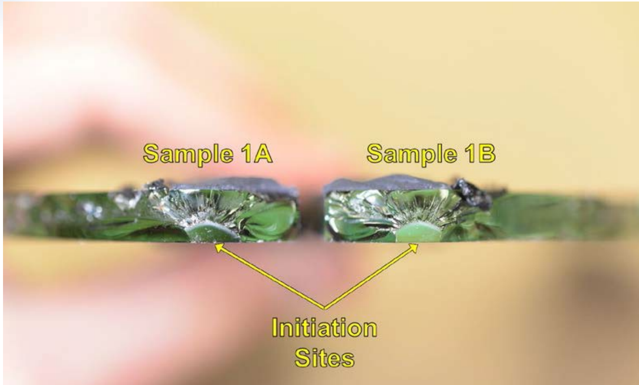
Fracture Origin Example-HS Glass with Ceramic Enamel
